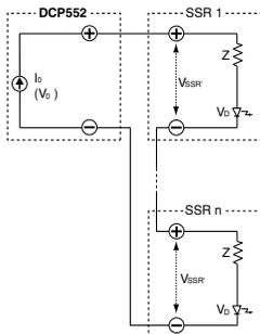
$$V_{SSR/MIN} \leq I_0 \times Z + V_D \leq V_0 / N \quad \text{Equation (3)}$$
