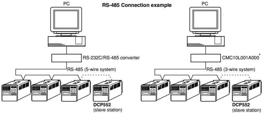
\* "Communication controller CMC10L001A000" is RS-232C/RS-485(3-wire system) converter in Azbil corporation.
