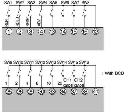
● Internal circuit diagram of the DCP552 connecting external switch input
