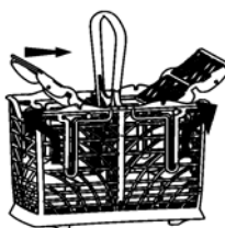
Movement required to extract the inserts
