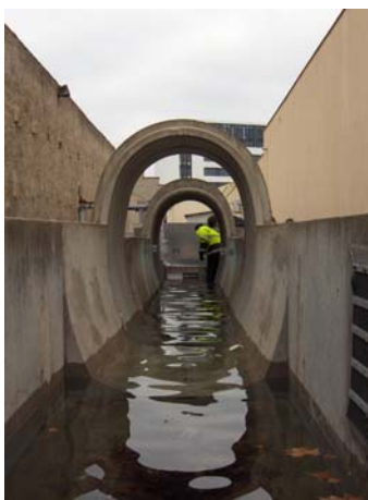
Figure 11. Experimental egg-shape sewer reach available at the Grand Lyon Sewer Dpt.
