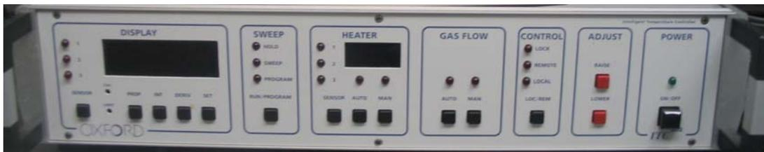
**Note:** The ITC controller has been preset by EMC staff for general usage. **Do not attempt to change the ITC setting.** If you do have a special need, contact the EMC staff for a change of setting.
