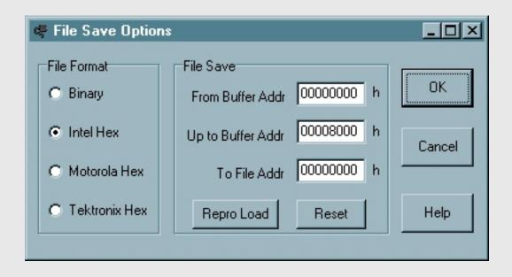
The File Save Options Dialog controls placement of data from Data Edit Buffer in the file as well as selection of the format in which the file is written(bin, hex, etc.). If a file has previously been saved, the File Save parameters will default to the previously entered values.
