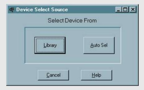
Click the AutoSel button to select the device by reading the device ID.
