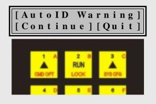
When the lower line on LCD displays text in brackets as in the above example , pressing the HOTKEY under the bracketed text will execute the command associated with the text.
