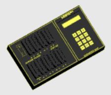
The Gangpro-8XP can operate fully autonomously to copy existing master devices...no PC is required. Up to eight target devices can be copied at once from one pre-programmed master device. No file downloading or master device loading to internal memory is required. The master device is copied to the target devices directly.
