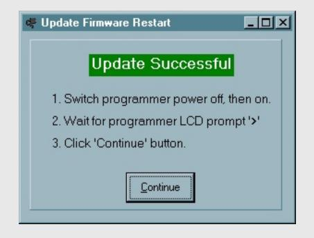
Turn off the GP-8XP as instructed, then turn it back on. Watch the display and make sure the version shown on the LCD matches the version of the update file. This completes the update process.
