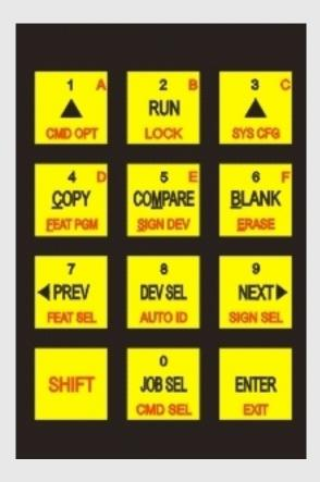
To execute key captions in red, Press and release [SHIFT],then press and release the red key.
