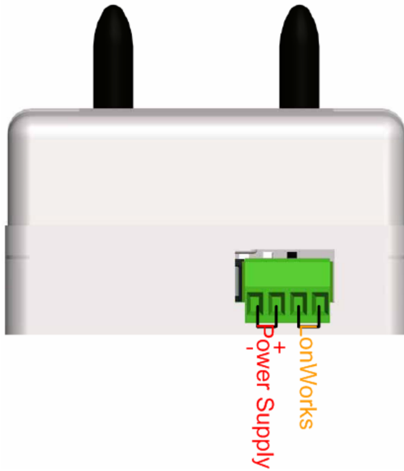
Figure 3.1 Connector pin assignment LonWorks network
