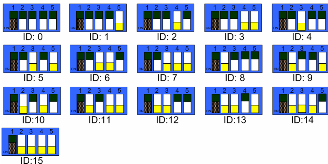
Figure 6.2 DIP Switch for Wireless network ID on 7600RF RF Receiver
