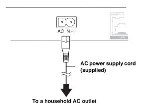
• This unit consumes a small amount of AC power ("Quick Start": "Off", approx. 0.1 W) even when turned off. In the interest of power conservation, if you will not be using this unit for an extended period of time, it can be disconnected.
