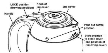
To remove the cover from the vacuum jug, turn it anticlockwise by means of the knob until the knob points to the symbol 'CLOSE', then take it out upwards. Reverse operation will refit the cover to jug,
