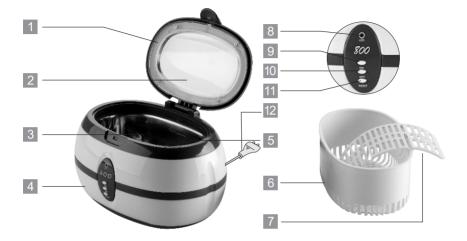
LID Z VIEW WINDOW STAINLESS STEEL TANK 4 HOUSING 5 "MAX"MARK PLASTIC BASKET PLASTIC WATCH STAND SINDICATION LIGHT ON"BUTTON O"OF"BUTTON 11 "RESET"BUTTON 12 PLUG AND CORD
