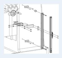
This option provides the machine operator positional feedback on the control when the knee is manual moved.
