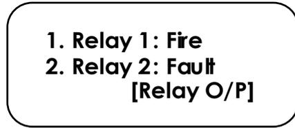
By selecting the number 1 in the keypad, it enters into the Fire Relay screen. It Displays as follows.
