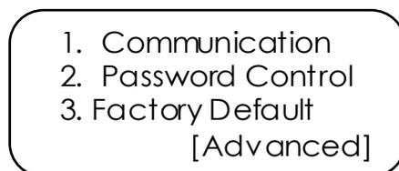
By selecting the number 1 from the Advanced screen, the system enters into communication mode. In this mode, network and repeater configuration can be done. After entering into this mode, screen will be as below.
