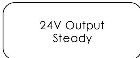
To change the option press '#' key to toggle between the options Steady and resettable.
