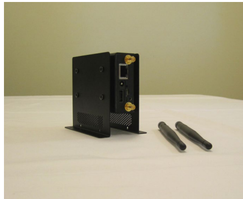
Figure 11. Kontron M2M System with 2x 802.11/802.15.4 Antennas
