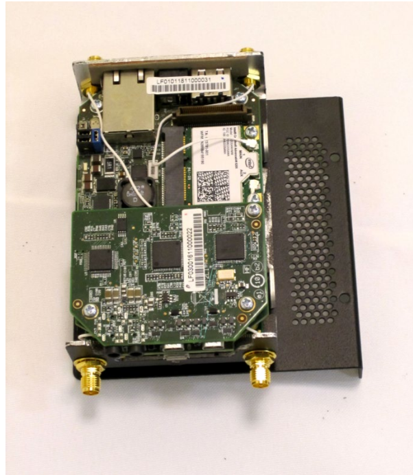
Figure 31. The Kontron M2M System with the 3G module fully installed
