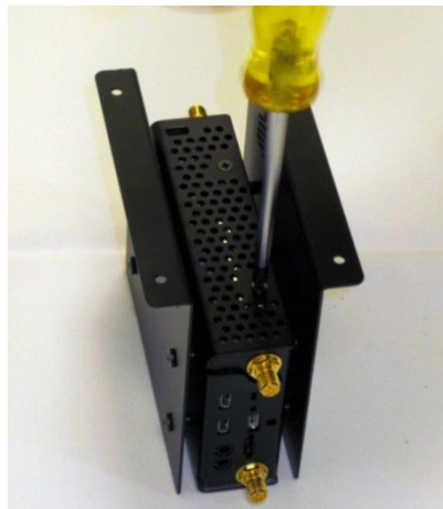
Figure 18. Unscrew the two bottom screws
