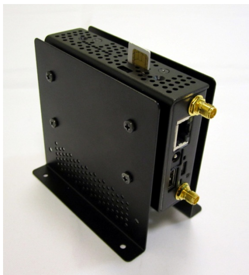
Figure 16. SIM Card Half-Inserted in the Kontron M2M System
