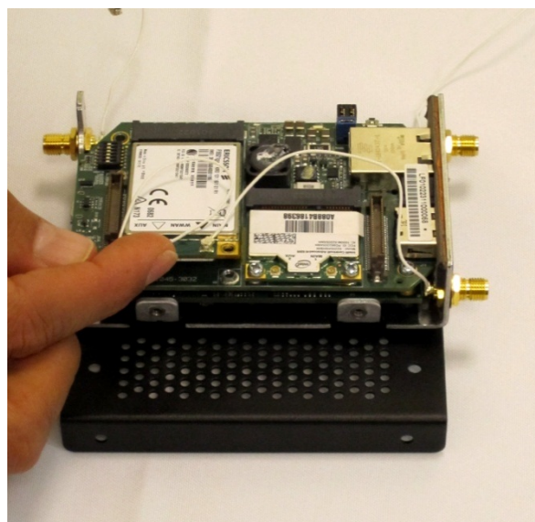
Figure 27. Position the module so that the screw holes are aligned
