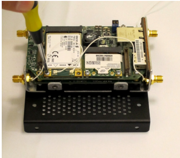
Figure 28. Screw the 3G module into place
