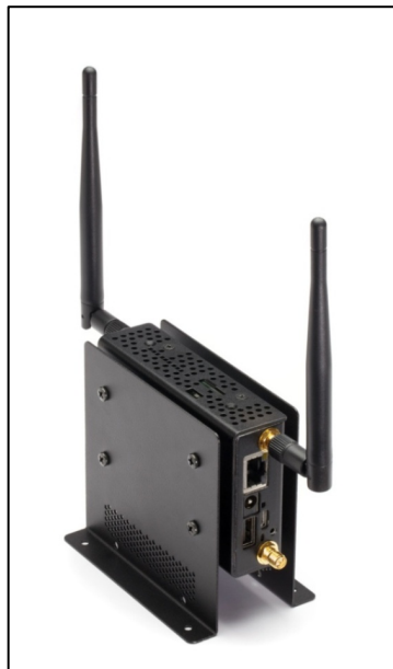
Figure 3. Kontron M2M System with 802.11/802.15.4 Antennas
