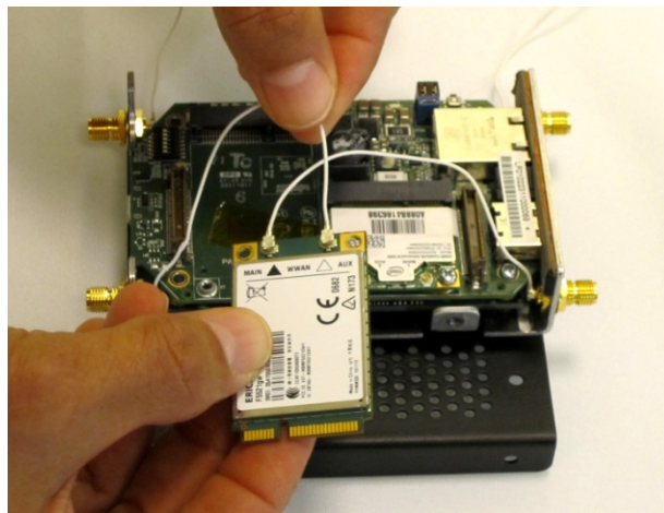
Figure 25. Attached 3G Module Card
