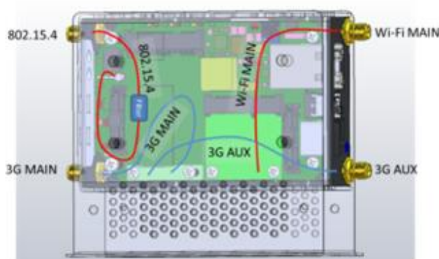
Figure 23. Antenna Cable Routing Supporting 3G Usage
