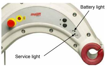
The electronics measures the operating time of the lifter, and after a specific time the yellow light will illuminate, indicating that the lifter needs service. Take contact with your local Molift service representative/dealer. The lifter can still be operated, but after a while an audible alarm will sound, to remind the operator that the lifter needs service immediately.
