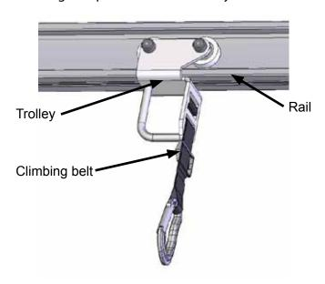
• Move the lifter until it stops at the end of the rail, and move the trolley on the opposite side as close as possible.
