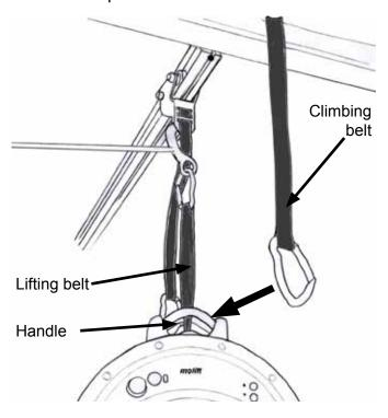
• Raise the lifter until it is possible to attach the climbing belt on the opposite trolley to the lifters handle.
