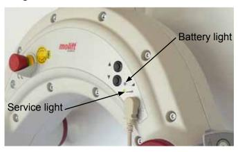
If the lifter is run up and down constantly for a longer period, the electronics may be overheated, and then the lifter will stop. The service diode will give a yellow flashing signal until the lifter has cooled down sufficiently to work again.
