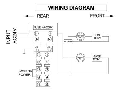
• Wiring Diagram (SHB-4300H1)
