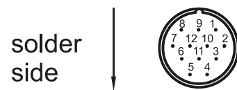
Fig.11: Viewing the RC series mating connector of the resolver (internal thread M23)
