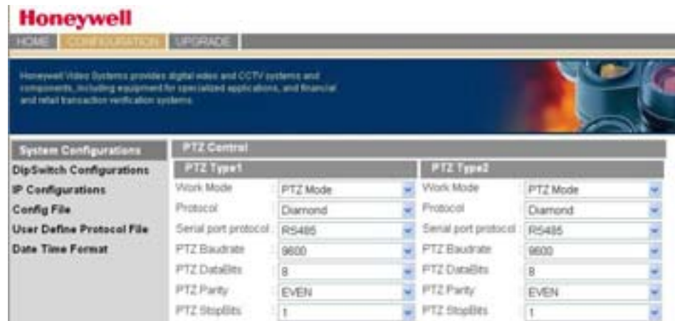
Figure 5-2 UART Port Setting Window
