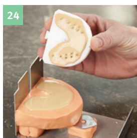
Invert the base plate onto the guide in the carrier plate and lower gently.
