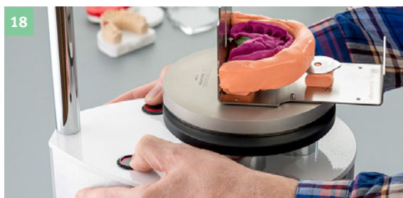
Press the button to start drilling – the plate support is held in place electromagnetically. WARNING: If the drill position/laser beam is outside the dental arch, then the burr may break, due to coming into contact with the plate support or the retention disc!
