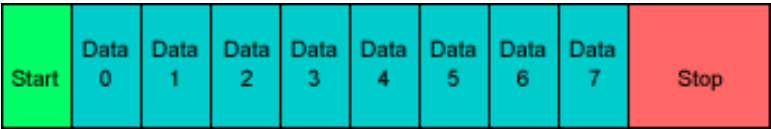
FIGURE 5.2: UART single byte frame
