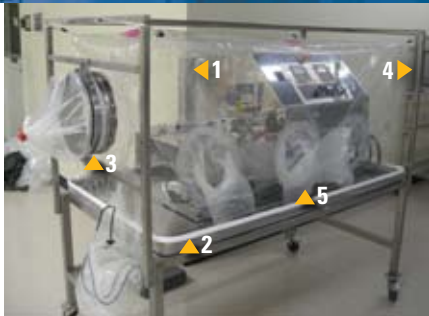
Figure 1 1 Enclosure 4 Support frame 2 Pan 5 Glove Sleeves 3 BIBO canister
