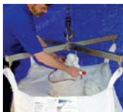
Securing the liner neck
