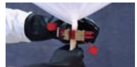
Squeeze tool until crimps are engaged -- then release tool
