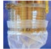
Canister and Transition Adapter Attached to ILC Dover Test Rig.
