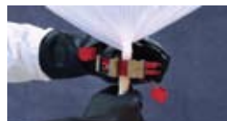
Squeeze tool until crimps are engaged -- then release tool
