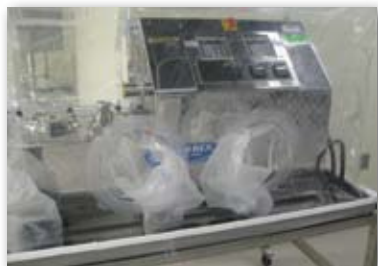
Solid Pan Mount Total Encapsulation Selected for Granulator
