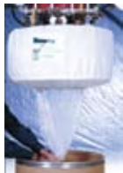
Sleeve is pulled into drum and filled
