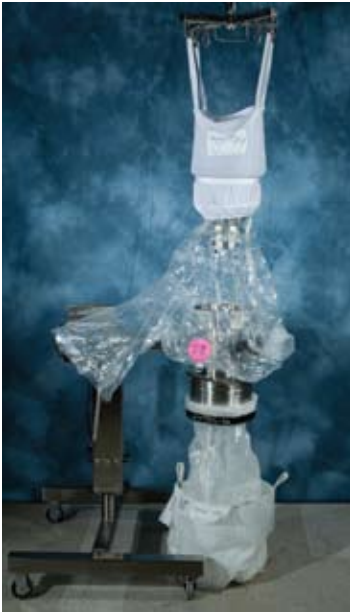
Figure 2. Shroud used to hoist canister.
