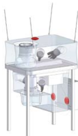
Overdrive Mill enclosure with shroud removed and fully deployed to allow use of glove sleeves for cleaning and maintenance
