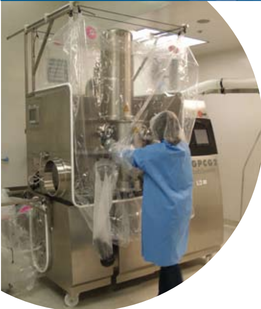
Fit check on lab scale fluid bed dryer
