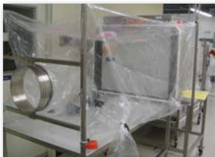
Flange Mount Flexible Containment Selected for Tray Dryer
