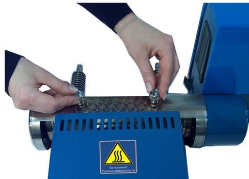
Fig.2-5 - Securing the thermal chamber unit on the external optical unit
