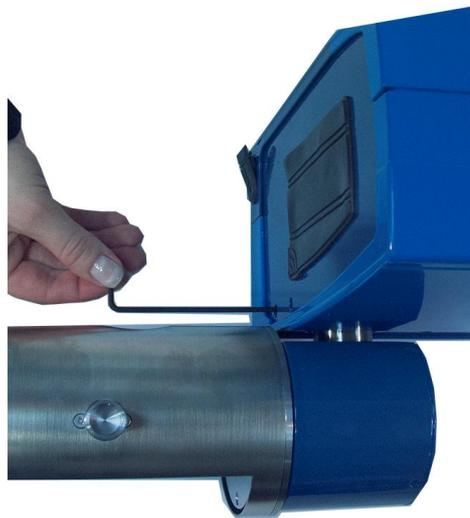
Fig.2-2 - Securing external optical unit on the mercury analyzer
