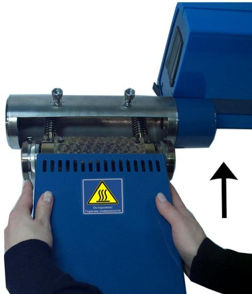
Fig.2-4 - Mounting the thermal chamber unit to the external optical unit
