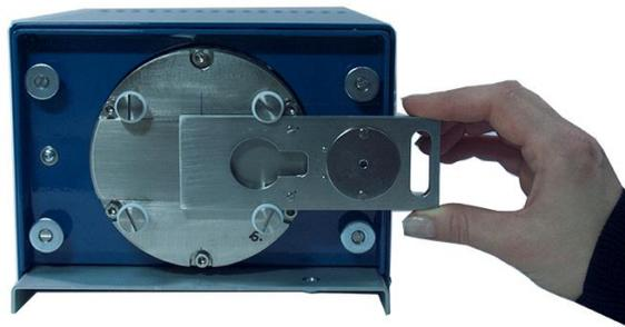
Fig.3-3 - Moving of the latch bar
