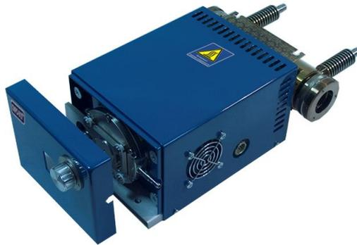
Fig.3-2 - Disassembling of the lid of the sample port
