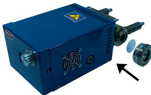
Fig.2-3 - Mounting quartz windows to the analytical cell
