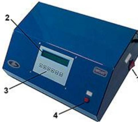
Fig.1-4 - Power supply and pumping unit (front side)
