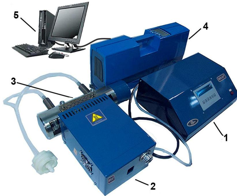
Fig.1-3 - The analytical complex (the RA-915M mercury analyzer with the attachment and the PC)
