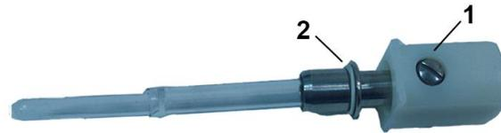
Fig.3-5 – The quartz boat with holder
