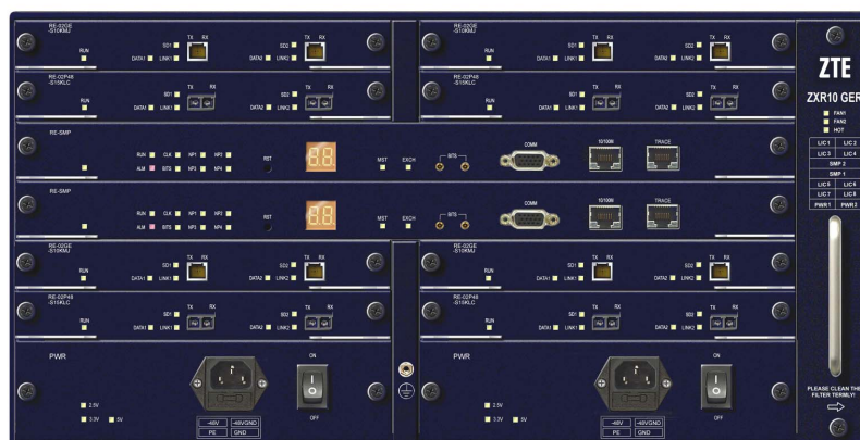
FIGURE 3 ZXR10 GER08 BACK PANEL VIEW
