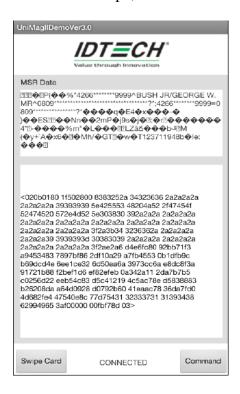
5. To send commands to UniMag, click on the button 'Command' and select the command to send.
