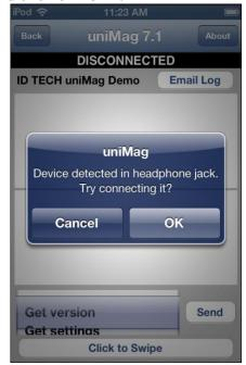
2. <Connecting with uniMag> message will pop up, as shown below. Make sure the reader status changes to <CONNECTED> after that.
