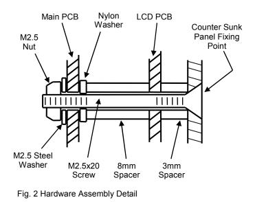
The countersunk head of the mounting screws are presented at the front of the LCD to support the mounting of the complete assembly to countersunk mounting holes within the chosen enclosure. The short nylon spacers provide clearance between the top side tracks of the LCD module and the rear of the mounting surface. The LCD header pins should be checked for clearance and if necessary trimmed to prevent contact with the underside of the enclosure surface.
