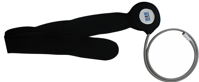
Figure 6. A, Inductive electrode without clamping band and B, inductive electrode with clamp band.
