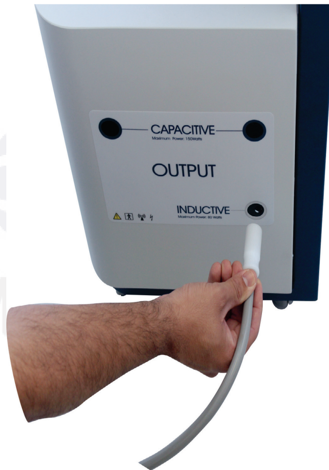
Figure 8. Installing the inductive electrode.
