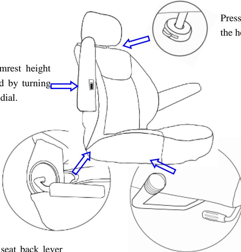
Press the bottom to adjust the height of the headrest.
