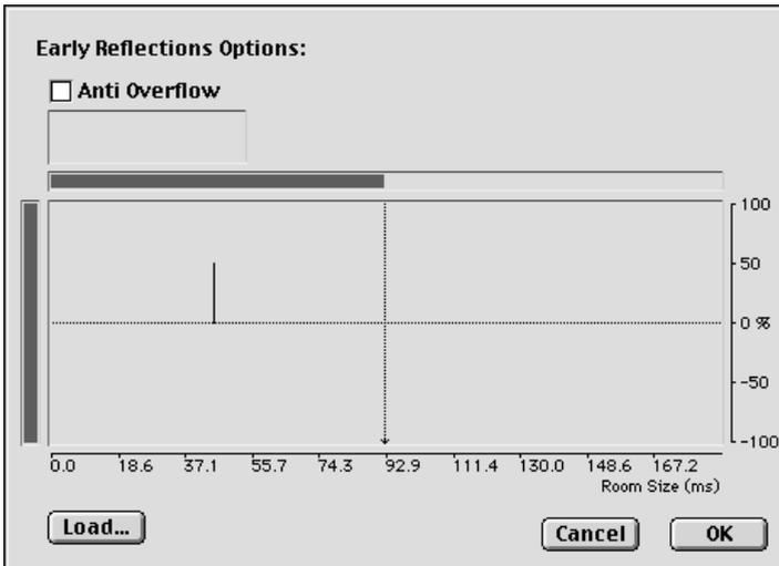
Double click on the module in Edit Mode or press **Opt** and click on the module in Run Mode to enter the Early Reflections Chamber's graphic edition screen. A vertical bar at the left allows you to adjust amplitude values on a percentage scale. A horizontal bar at the bottom enables you to mark the length of the early reflection effect (timewise). You are therefore selecting the room size. To edit these two bars, click and drag with the mouse and adjust.
