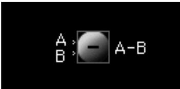
Please remember that the signal to be subtracted must be inserted into the second input, as can be seen in the figure above.
