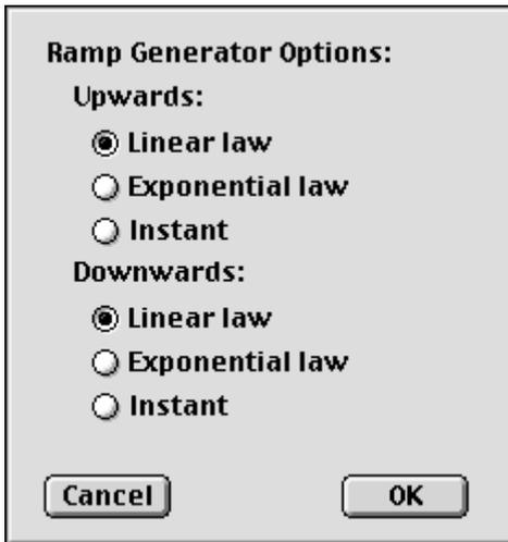
**Linear:** The generated signal between two points is a straight line which joins them.
