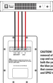
**CAUTION!** Requires removal of terminal cup and cutting of both the yellow and the blue jumper wires that connect the SPK1 and SPK2 terminals.
