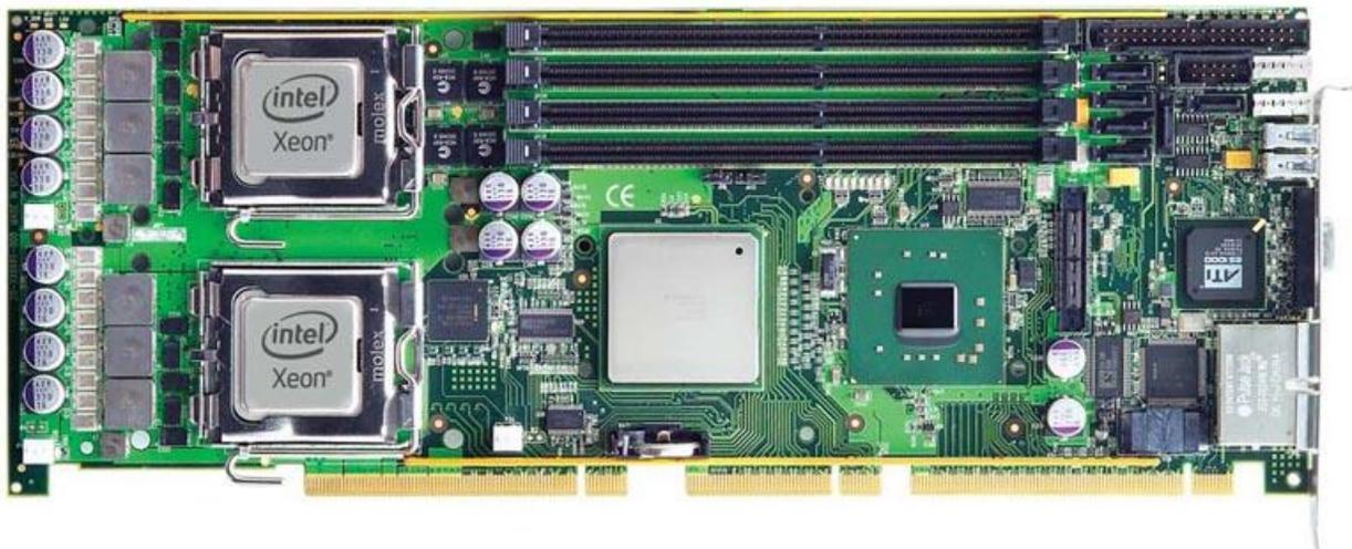
Figure 6-5 Trenton PICMG 1.3 Sys/Host Board
