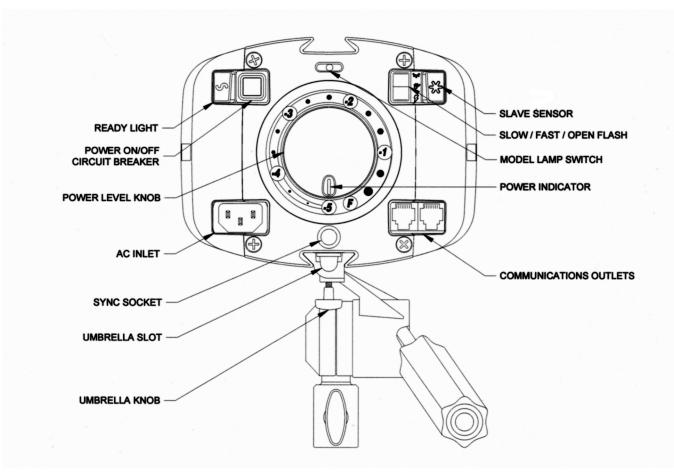
• **POWER ON/OFF / CIRCUIT BREAKER** Overload protection is built into this push button switch. If an overload should occur, the button will pop out to the Off position.
