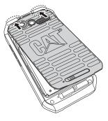
3. Push the back cover firmly to secure it into place.
