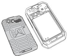
2. Engage the hooks on the top of the back cover with the designated holes on your phone.
