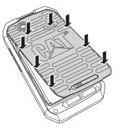
4. Press and hold the bottom of the back cover and slide the back cover latch to the left to the lock the back cover.
