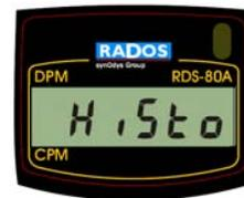
Press the push button shortly to return to the main menu or wait 7 seconds to return to the dose rate display.
