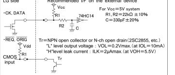
Since the power voltage differs between the gage side and an external device side, absolutely use an open collector or open **CAUTION** drain circuit. Do not use a CMOS output, etc.
