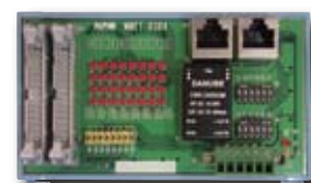
MNET-304 Local Output Board (Isolated 32 outputs)
