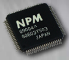
G9004A Local Device CPU Emulator
