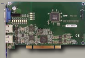
PPCI-L112 PCI Bus Center Board (G9001A x 2)
