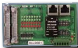
MNET-322 Local Input/Output Board (Isolated 16 inputs/outputs)
