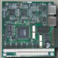
NPMCMNET-I/O104 PC/104 Bus Center Board (G9001A x 2)
