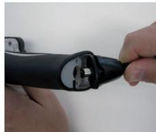
3. Press the 8-pin DIN plug and protective cap onto the socket.
