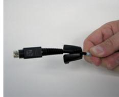
2. Align the 8-pin plug so that it fits into the socket on the handheld.
