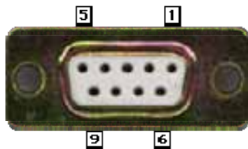
Figure 5-5: RS-232 Touch Panel Connector
