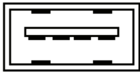
Figure 5-6: USB Touch Panel Connector
