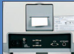
Circuit points on the rear: Printer, keyboard and VGA-monitor
