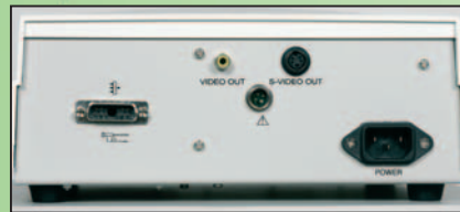
Connectors to archiving systems by video-out and S-video-out
