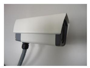
11. Finally, the box camera with properly mounted flex conduit as well as with proper outdoor bracket would look like this.
