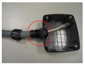
7. Connect the flex conduit to the back side cover of the camera.
