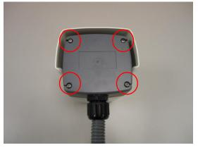
10. Tighten the screws of the back side of the camera properly.
