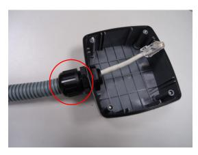
8. Tighten the domed sealing nut.
