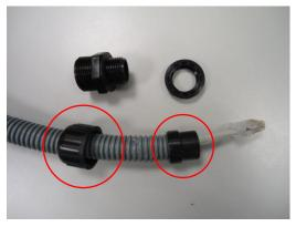
3. Two pieces from the conduit gland set will be attached to flex conduit first.
