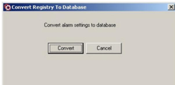
Converts the alarm settings from the Registry to the new format and adds the computer name. It only converts settings for SMS, Minicall and relay outputs. Click **Convert** to start the conversion. Click **Cancel** to close the dialog.
