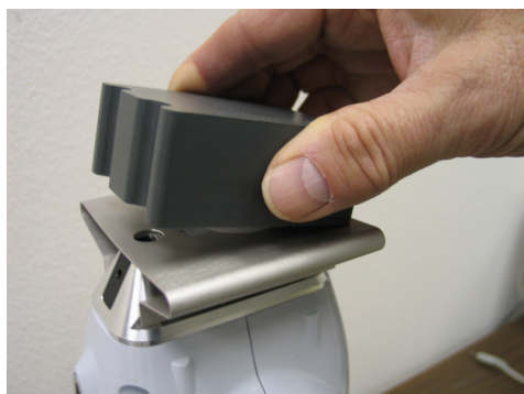
Figure 4.17 Preparing to use the safety shield when testing a very small sample. The safety shield must be completely flat against the sample holder with the instrument IR sensor covered for testing.
