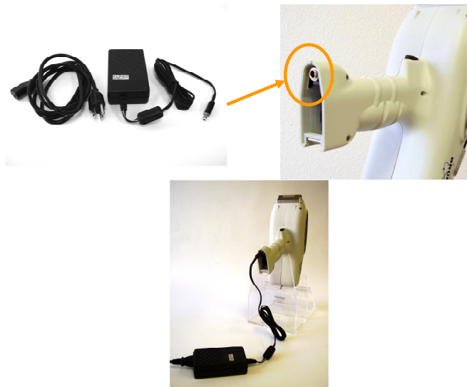
Figure 4.3: Operating the S1 TRACER using AC power
