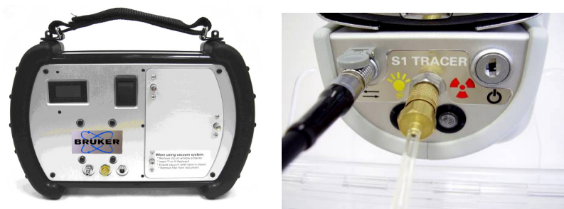
Figure 4.11: Attaching the vacuum tubing
