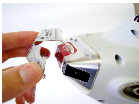
Figure 4.13: Installing/removing the clip-on window protector
