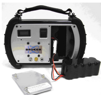
Figure 4.8: Removing the battery from the vacuum pump
