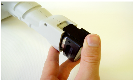
Figure 4.1: Removing the battery from the S1 TRACER
