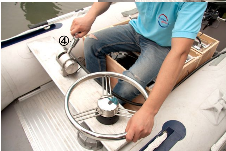
④:Put backward the remote speed control joystick set,so that the boat will go backward
