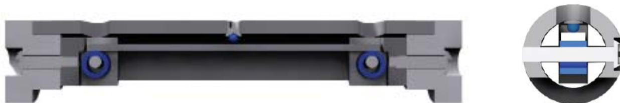
Cutaway of Bent Beam Coupon Holder With Coupon Installed
