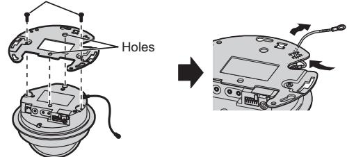
9. Attach the connector cover (included) and connect the necessary cables to the camera.
