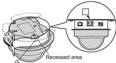
10. Attach the camera to the bracket in 3 places using screw B (included).
