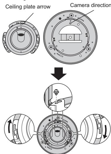
11. Secure the ceiling mounting cover (included) to the bracket.
