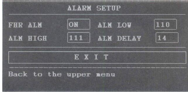
Figure 3.6 Alarm Setup
