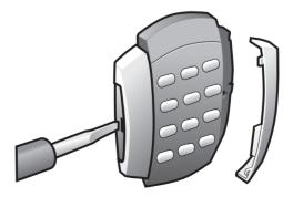
To release Security Caps push a screwdriver into slots on the side and pull forward.
