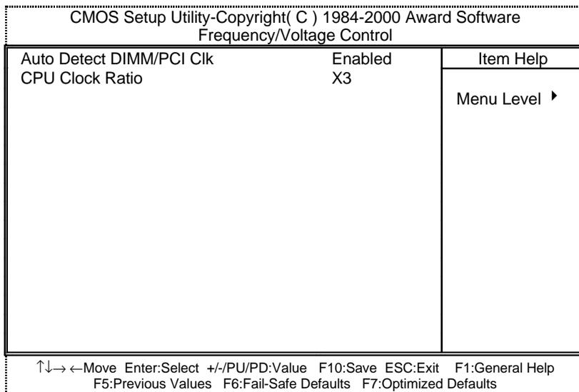
Figure 10: Frequency/Voltage Control
