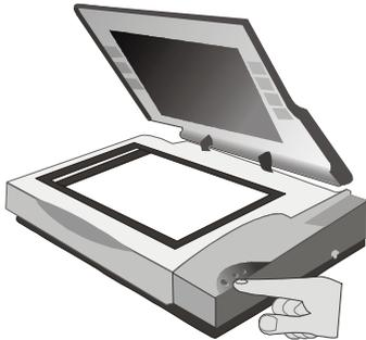
The LED power indicator on the front panel of the scanner lights up and flashes for about a minute and then remains lit, signifying that the scanner is ready.
