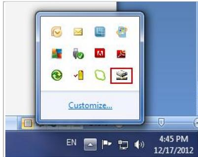
If EN-V-R is not running, you can go ahead to next section of uninstalling the program. If EN-V-R is active, place the mouse pointer on the EN-V-R icon, and click the right mouse button. You'll see the pop-up menu. Select **Exit**.
