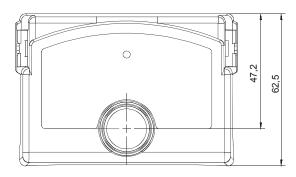
LMO... with extension of lockout reset button AGK20...
