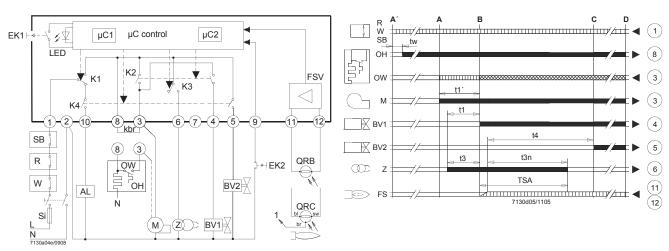
AL Alarm device BV... Fuel valve
