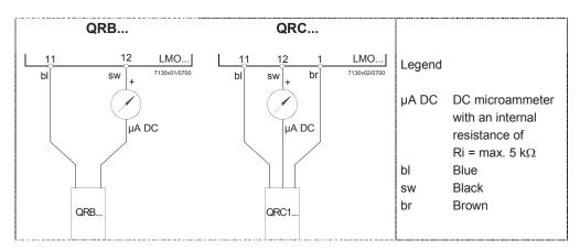
As an alternative to detector current measurement, the Interface OCI400 / with PC software ACS400 / ACS410 can be used. In that case, the DC microammeter is not required.
