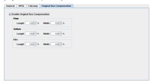
It is possible to specify the magnification of x-direction and y-direction independently for each media.
