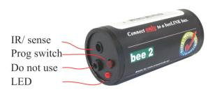
**The IR/ sense** socket is output for the IR-emitter that sends IR to the device to be operated. In some cases this socket is also used for sensing purposes. Sometimes the BeeLINK2 controller needs to know if the device is powered up or not.
