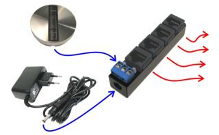
A Bang & Olufsen IR-receiver connected to the BeeLINK link amplifier with four BeeLINK outputs.
